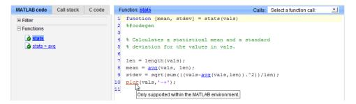
For unsupported functions other than common visualization functions, you must declare the functions (like pause) to be extrinsic (see "Resolution of Function Calls in MATLAB Generated Code" on page 13-2). Extrinsic functions are not compiled, but instead executed in MATLAB during simulation (see "How MATLAB Resolves Extrinsic Functions During Simulation" on page 13-16).
