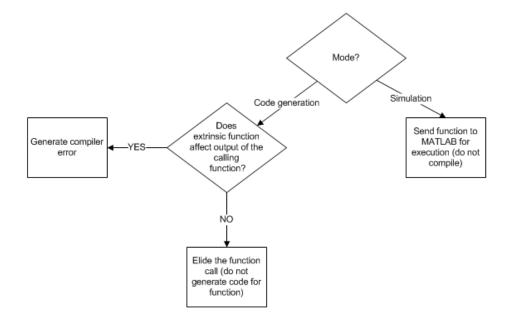
During simulation, MATLAB generates code for the call to an extrinsic function, but does not generate the function's internal code. Therefore, you can run the simulation only on platforms where you install MATLAB software.
