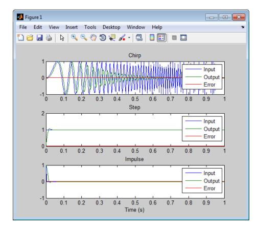
**4** Optionally, zoom in on each plot in turn to view the error (difference between the two versions of the algorithm). In this example, the errors are very small, on the order of  $10^{-3}$ . If the error is unacceptably large, refine the fixed-point data types.
