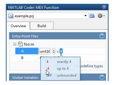
**5** From the list of size options, select :4 to specify that the second dimension is variable size with an upper bound of 4. Alternatively, select :Inf to specify that the second dimension is unbounded.
