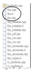
**Note** If you specify C++, MATLAB Coder wraps the C code into .cpp files so that you can use a C++ compiler and interface with external C++ applications. It does not generate C++ classes.
